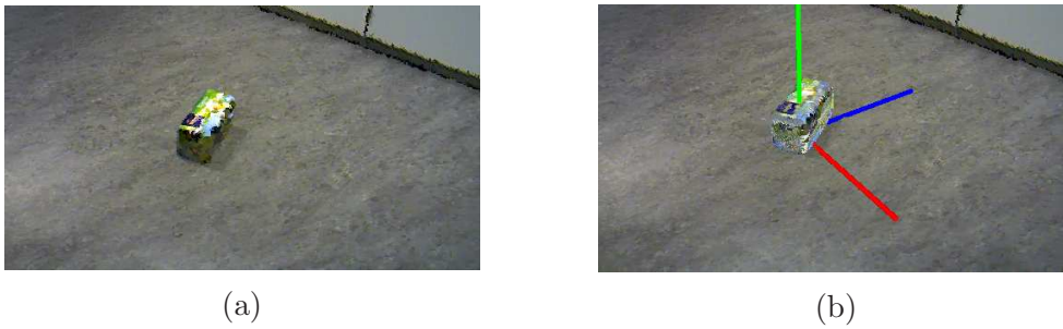
Figure 6.2: Original object (a) and superposition of the recognized object in its estimated pose with the real scene (b).
