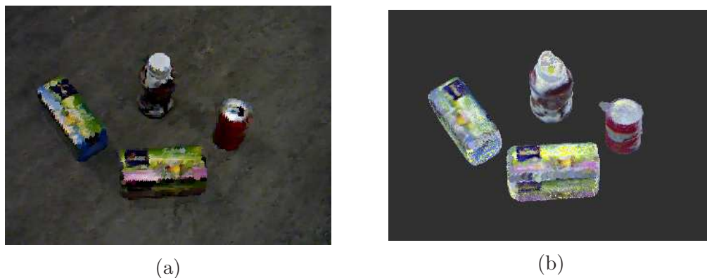
Figure 6.3: Original camera view (a) and reconstructed 3D models based on the estimated poses of the recognized objects (b).
