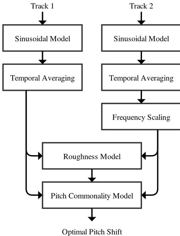
Figure 1: An overview of the proposed approach for consonance-based mixing.
