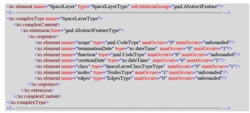
Figure 26 - Semantic attributes stored in SpaceLayer features as per IndoorGML v1 XSD Schema (OGC, 2014)
