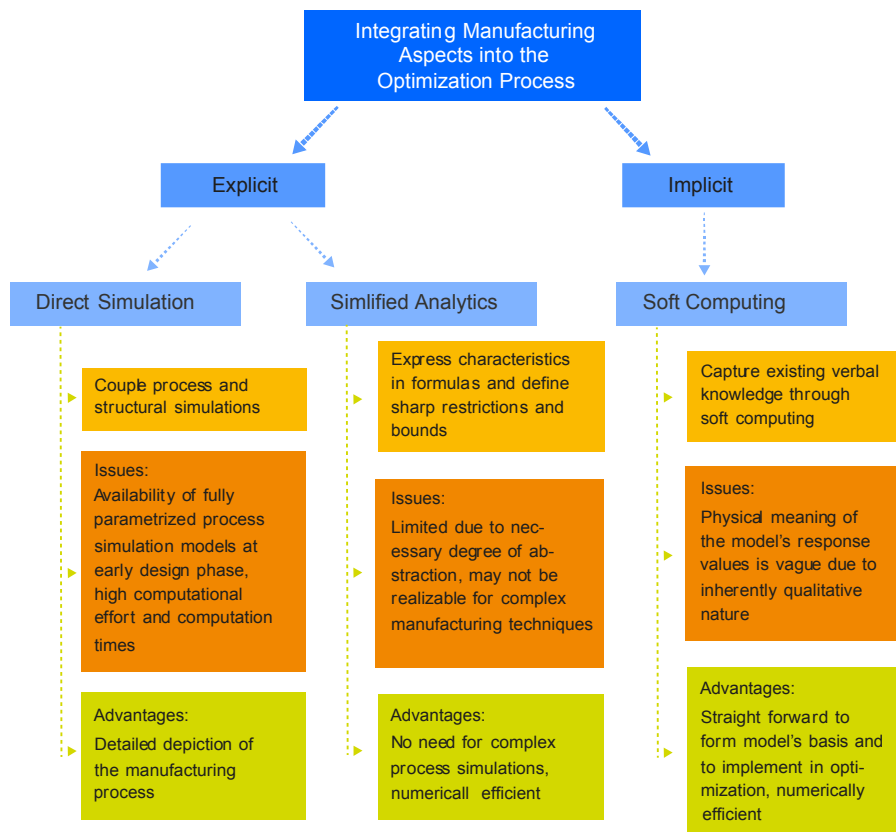
Figure 4.1.: Categories for modeling manufacturing aspects such that they can be introduced into the optimization process
