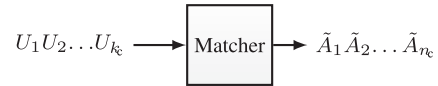
Fig. 7. The matcher transforms uniform data blocks of length k_c into n_c amplitudes that are approximately distributed according to the desired distribution P_A . By replacing the amplitude source P_A in the PAS diagrams in Fig. 3 and Fig. 5 by a matcher, our scheme provides a binary interface to the source coding part of a digital communication system.
