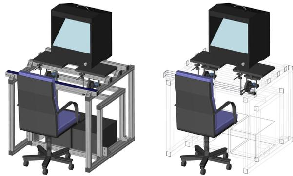
Fig. 2. **Master console with PHANTOM devices and 3D screen**
