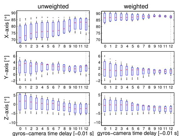
Fig. 9. These box plots show the performance of the unweighted and weighted rotation estimation on not correctly temporally aligned real data. The black dotted line corresponds to the mean of the estimated delays between camera and gyros of all runs.
