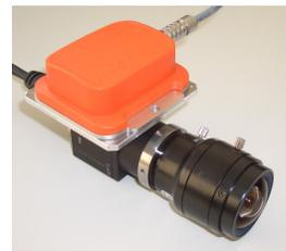
Fig. 1. A PointGrey Flea2G camera with wide angle lens and a Xsens-MTi IMU (orange box) as it is used in our experiments.
