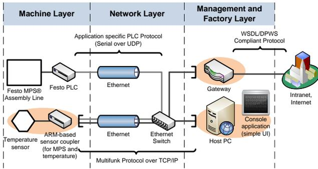
Figure 2. Network Structure in the Use Case
