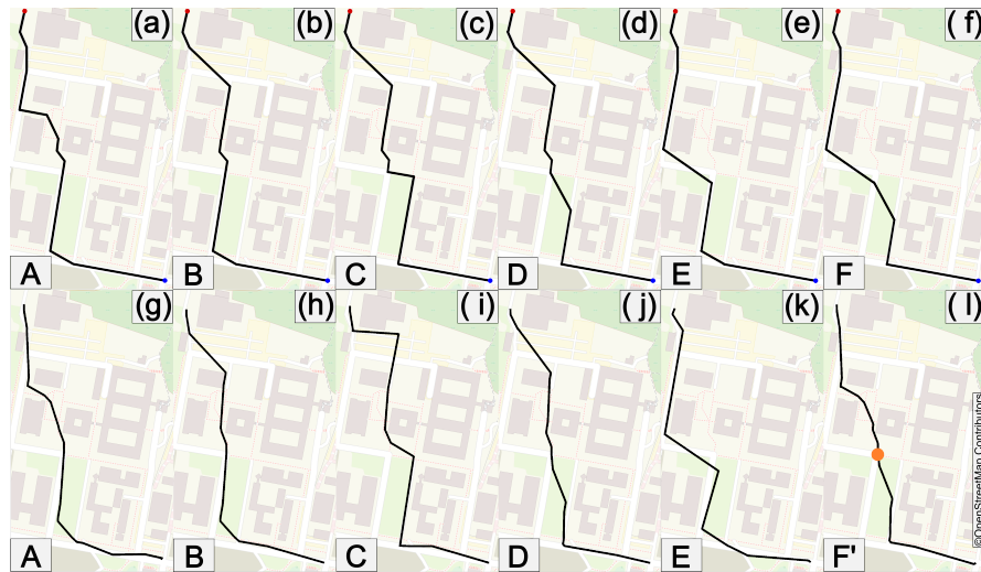
Fig. 3 (a) - (f): The measured walking routes of the festival visitors A to F. (g) - (l) show the simulation walking routes A to F'. The orange marker in (l) indicates the falsely predicted route choice. All routes start at the bottom and end at the top. An extended version of the graph-generation method of [9] was used for the case study scenario.
