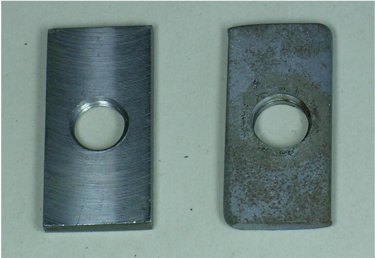
Fig. 29: LCPC impeller before (left) and after (right) test run, indicating the abrasiveness of the material.
