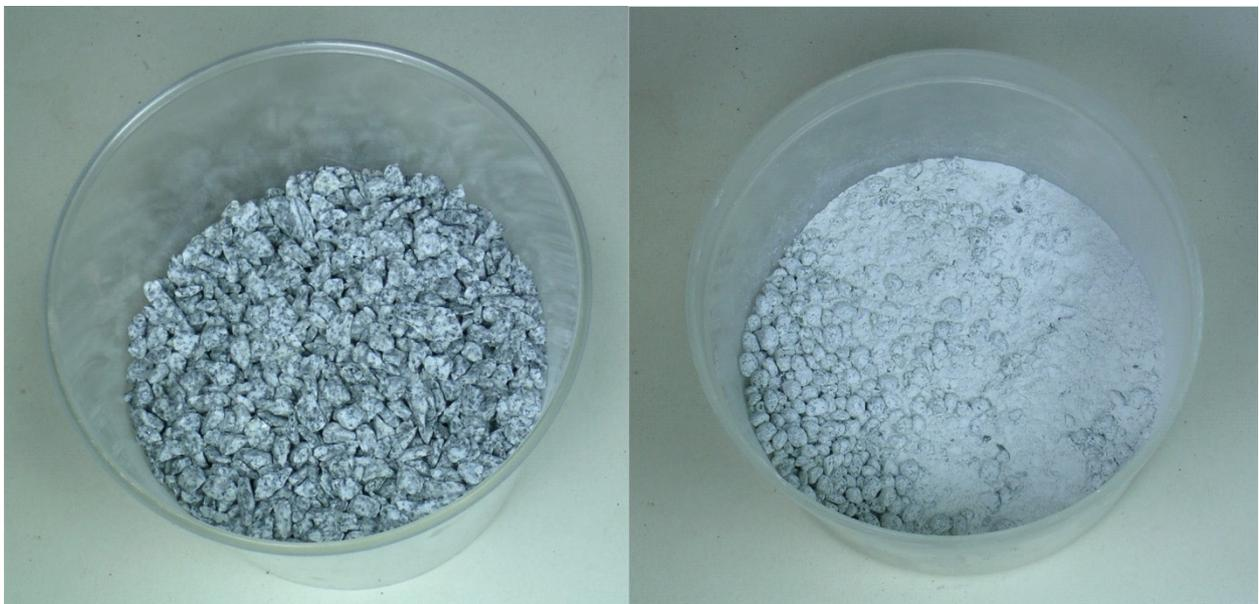
Fig. 30: LCPC sample before (left) and after (right) test run. The grain size ranges between 4 and 6.3 mm before testing.
