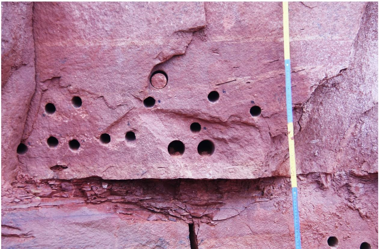
Fig. 38: Exemplified drill pattern and bore holes for rock sampling in the quarry of Miltenberg.
