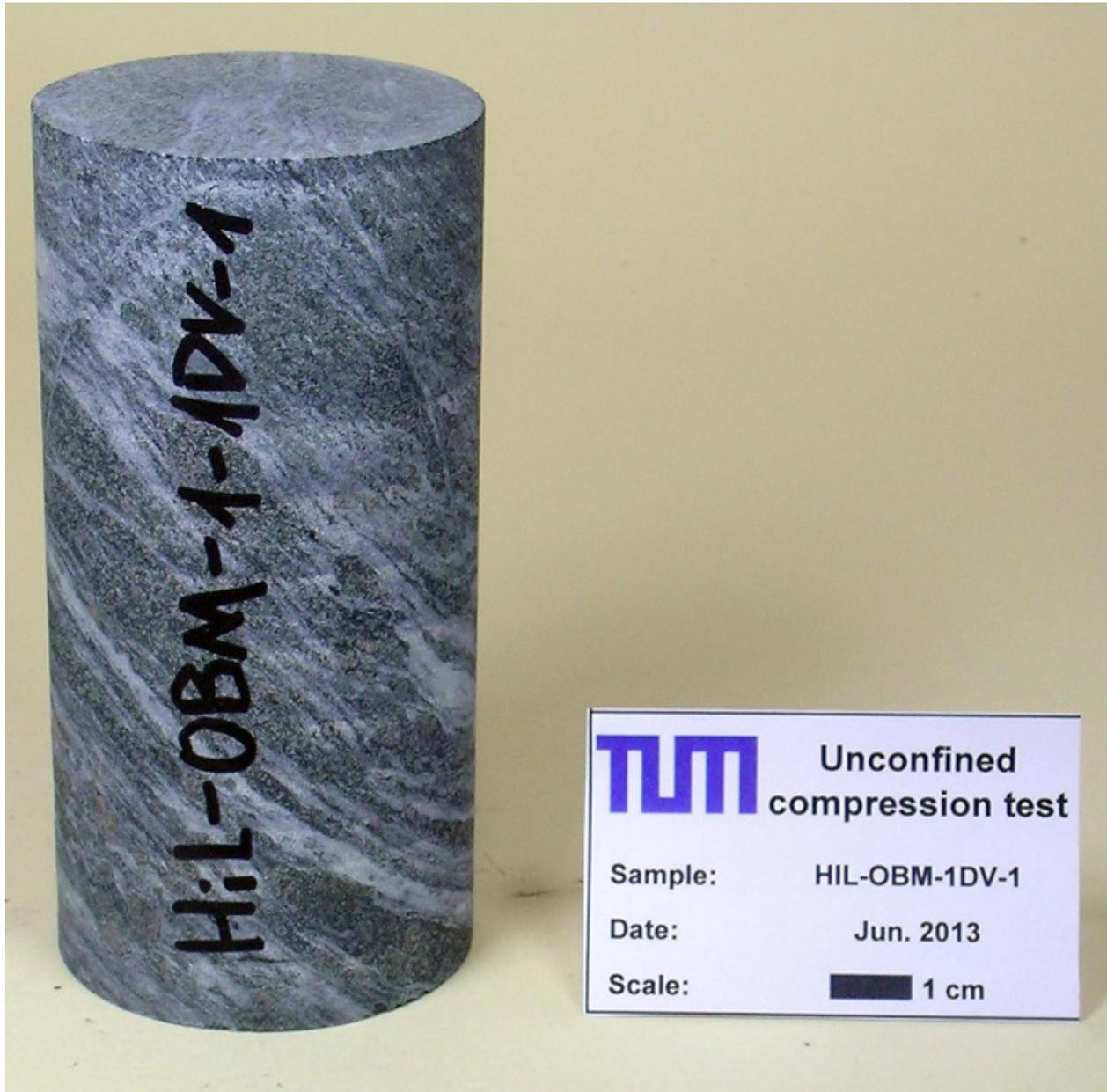
Fig. 62: Picture of the UCS sample of amphibolite of quarry Oberbaumühle. HIL-OBM-01.
