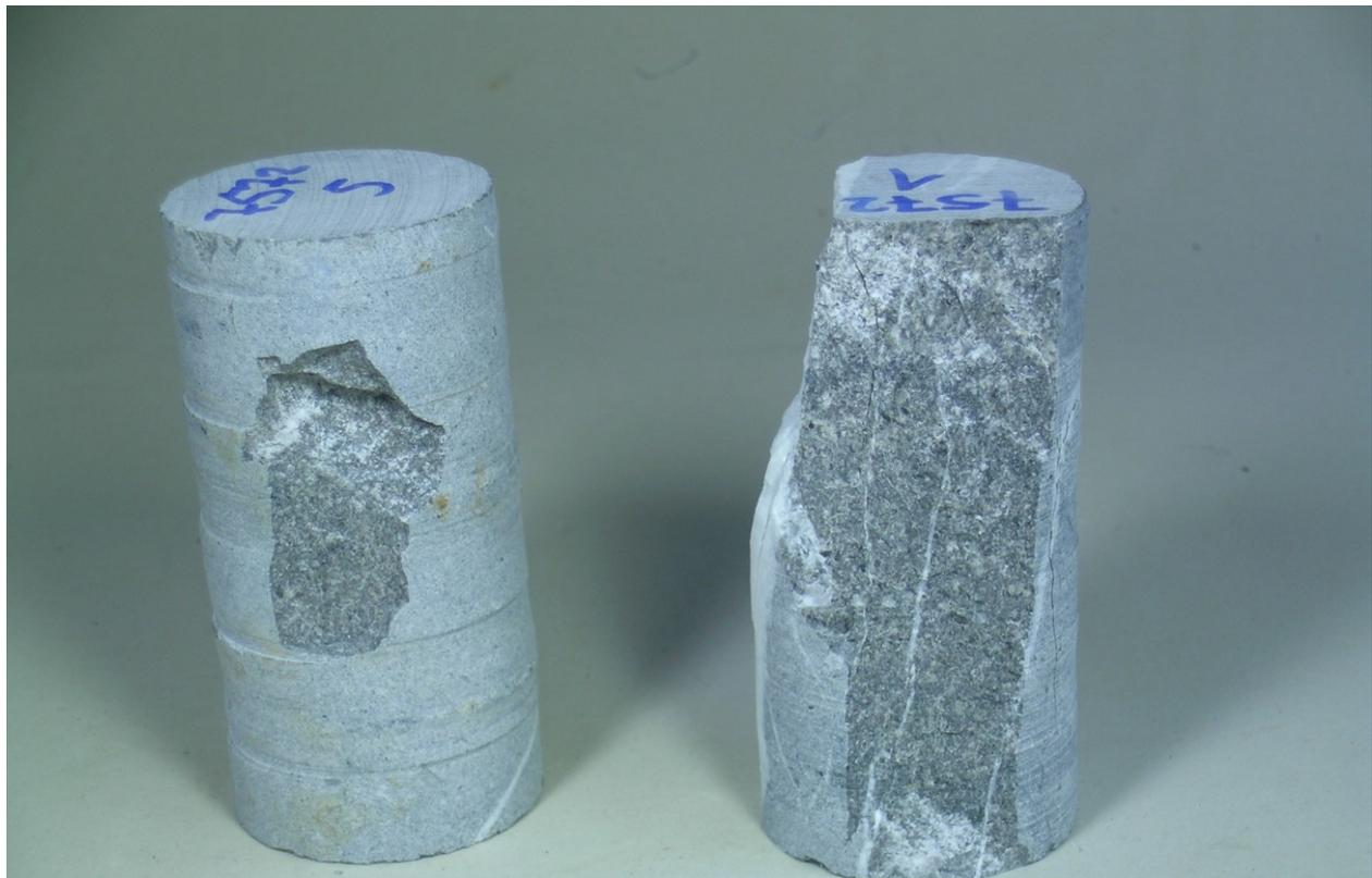
Fig. 59: Picture of UCS samples of the siliceous limestone of Hagerbach Test Gallery.
