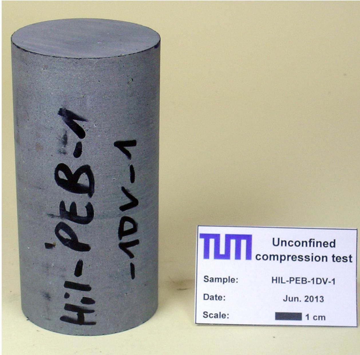
Fig. 64: Picture of a UCS specimen of the Pechbrunn basalt. HIL-PEB-01.
