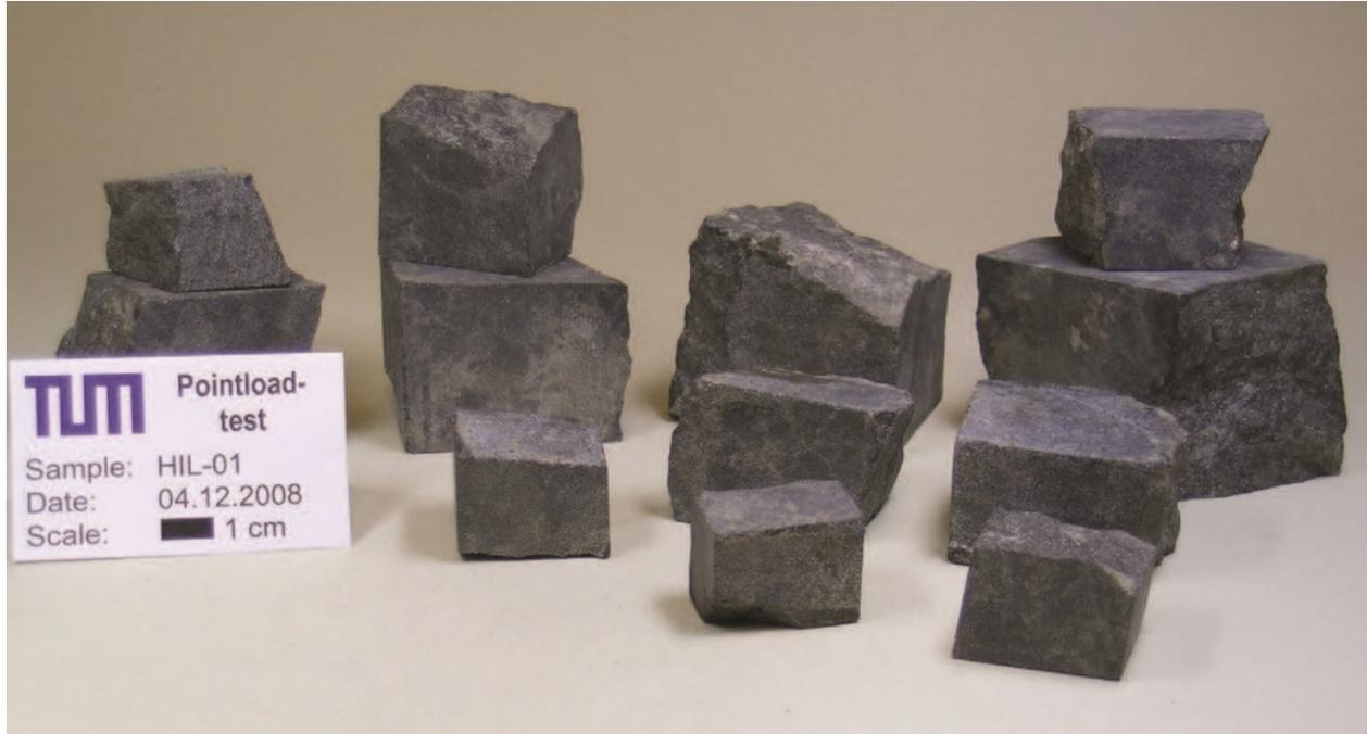
Fig. 43: Specimen of anorthosite for the point load testing of Blue Ridge mine.
