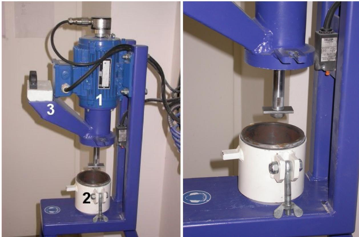
Fig. 28: Left: Abrasimeter with a 700 W electric motor (1), sample container (2) and funnel tube (3) for the filling of the sample container (closed during operation). Right: Mounted metal impeller, which rotates with a speed of 4500 rpm for 5 minutes through the sample.
