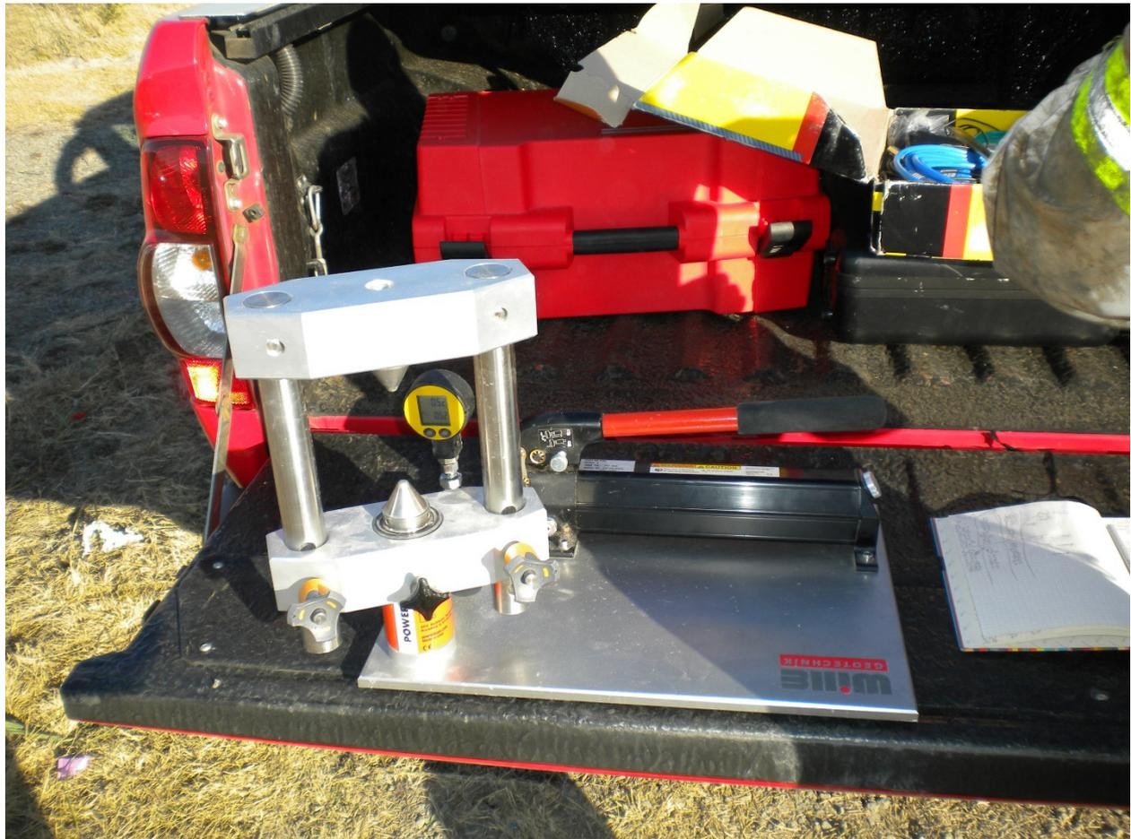
Fig. 23: Illustration of the point load field testing device: Left load frame including the test cones; right hydraulic manual pump (Picture: Johan Fourie).
