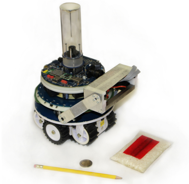
Fig. 2. The marXbot robot with its manipulator, and, on its right, a compliant pocket.
