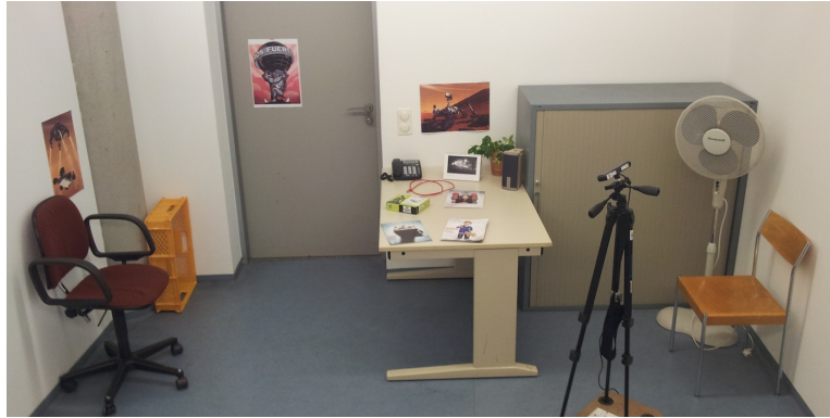
Figure 5.5: Office scene used for the evaluation of transparency detection. Transparent objects are placed on the table, and the tripod with an Xtion depth sensor (right) is then moved around the table.
