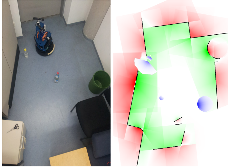
Figure 3.11: An office scene is mapped by naïve haptic exploration and fitting of geometric primitives. Occupied areas are depicted in red, free areas in green and movable objects in blue. Color intensity corresponds to mapping confidence. Figure adapted from [5].
