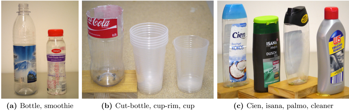
Figure 6.9: Real objects used in the experiments for haptic exploration and classification. Four plastic cups in (b) were put into each other, since the force sensor was not sensitive enough for a single one. The cut bottle also belongs to the “cup” class. Bottles in (c) all belong to the “elliptic” class. Figure adapted from [9].
