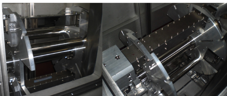
Figure 9: The revolver polarizer changer between (left) a plain neutron guide segment and (right) the polarizer. The two remaining positions have been left for further options.
