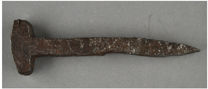
Figure 3: A Celtic nail from the oppidum of Manching (ca. 9 cm long) containing only 37 ppm of Cl after thermal treatment in welding gas (N 2 + 10 % H 2 ) at 750 °C. The treatment took place 25 years ago and the nail survived with hardly any corrosion. PGAA shows that it contains only 37 ppm of chlorine.
