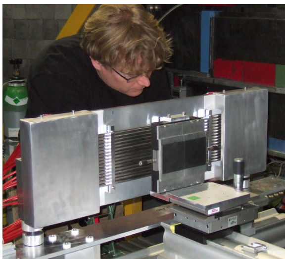
Figure 5: A module with 16 position sensitive ^3\text{He} -tubes destined to be used at SAPHiR during a test with collimated neutron beam at TREFF. Currently, the qualification of all tubes and the corresponding readout electronic modules recently arrived as well as the mechanical design of the detector is in progress.
