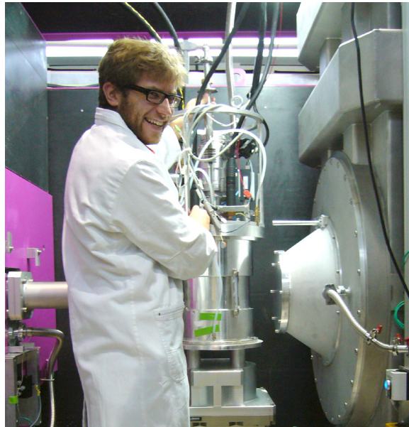
Figure 3: Setting up the vacuum furnace for high temperature measurements at SANS-1 instrument.
