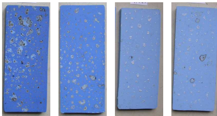
Figure 41. Samples of filler A2 without standard grade ATH (120 x 50 mm) at 1 wt% and 3 wt% and containing ATH at 1 wt% and 3 wt% (from left to right) after UV and acid stress.
