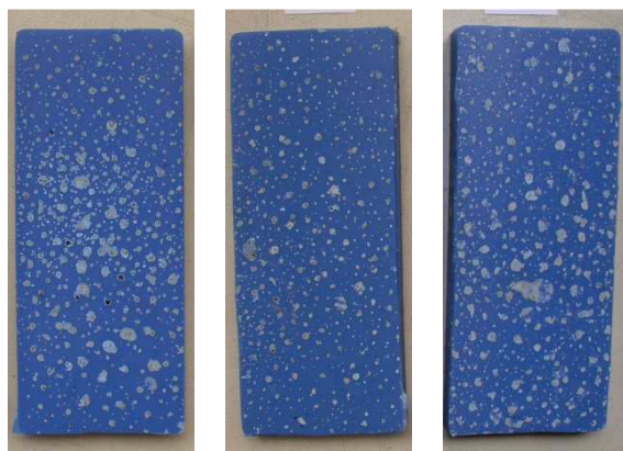
Figure 39. Samples of filler A1 without standard grade ATH (120 x 50 mm) at 1 wt% (left), 3 wt% (middle) and 5 wt% (right) after UV and acid stress.
