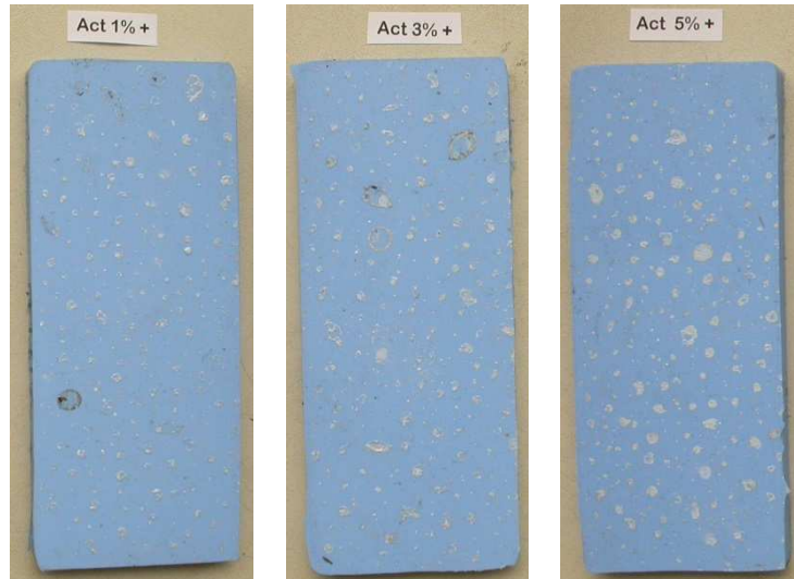
Figure 43. Samples of filler A3 containing standard grade ATH (120 x 50 mm) at 1 wt% (left), 3 wt% (middle) and 5 wt% (right) after UV and acid stress.
