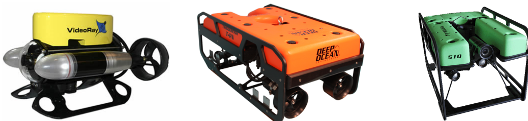
Figure 2.3: Underwater Remotely Operated Vehicles ROVs: ROV from the Marine Technology Society (left)[Mar12], T4N ROV (center) and L4N ROV(right) from the Deep Ocean Engineering, Inc. [Dee14]
