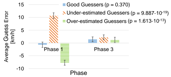
(b) Influence of learning effect on guess error of speed perception [Tan13c]
