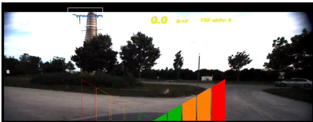
(b) Operator interface with additional information for the operator for a critical situation
