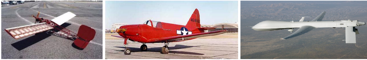
Figure 2.2: Radio-controlled target drones. Radioplane RP-5A (left) [Fon01a, p. 124], Culver PQ-14 (center) [Fon01a, p. 124] and US Air Force Predator (right) [Gen14]
