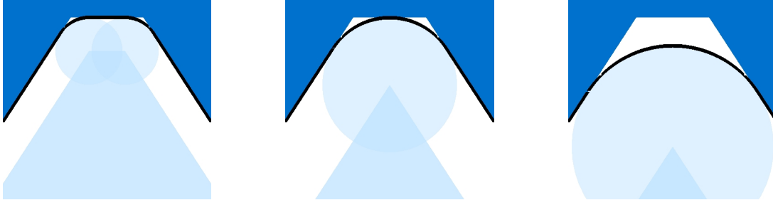
Figure 5.6.: Details of sample shapes to demonstrate the effect of pure rounding (from left to right) or de-rounding (from right to left) while the shape is drawn with a bold black line, the circumscribing polytope is represented by the boundary of the blue area, the angular light blue area highlights the kernel polytope and the light blue circles illustrate the radius \lambda_r
