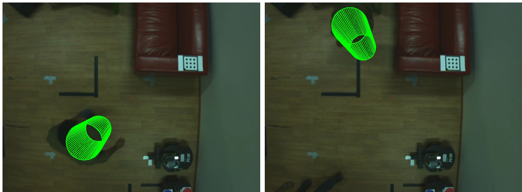
FIGURE 2.21: Illustrating the monocular MCMC tracker. Here, the rigid cylindrical shape model is visible, which is used as a coarse but sufficiently approximated representation of the human body, as it is observed from a supracranial perspective.
