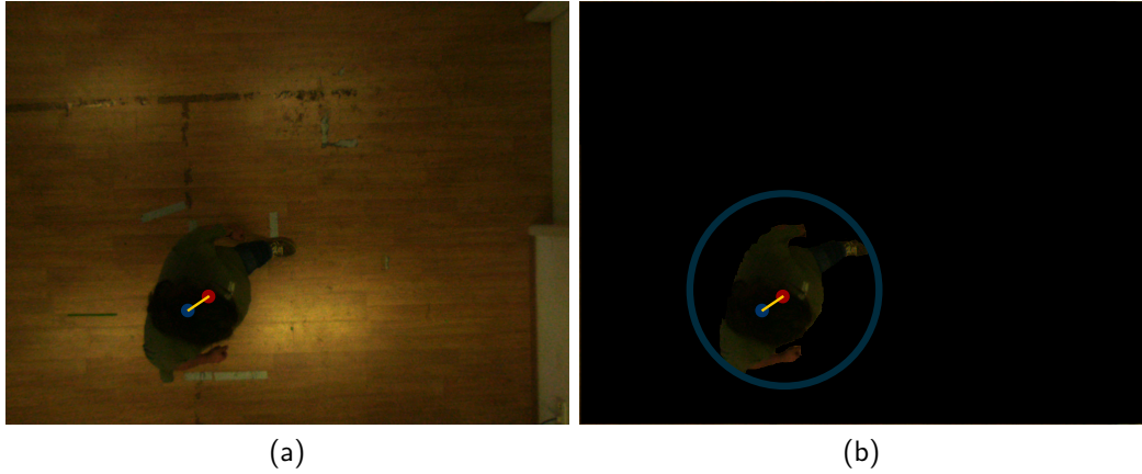
FIGURE 2.30: Illustrating the error metrics used to evaluate single-view tracking performance. (a) depicts the absolute tracking error d_a (yellow), measuring the distance between ground truth position (red) and candidate position (blue). (b) depicts the current circumcircle of the target blob (turquoise), used to calculate the relative tracking error d_r .
