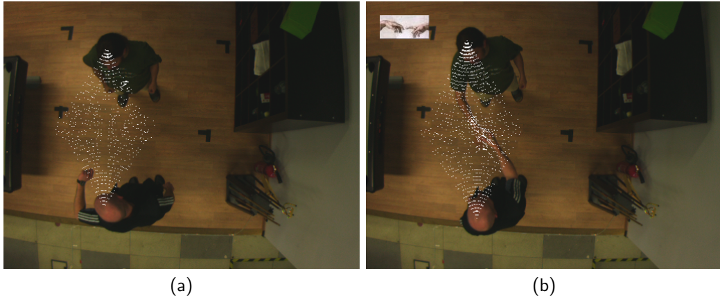
FIGURE 4.1: Two persons shaking hands, as seen from a supracranial perspective. In (a), the optical flow fields extending from the tracked pedestrian positions towards each other can be seen, before the handshake occurs. In (b), the handshake has occurred and was detected by the system, which is signified by the icon in the upper left corner in the display unit for human-readable output.
