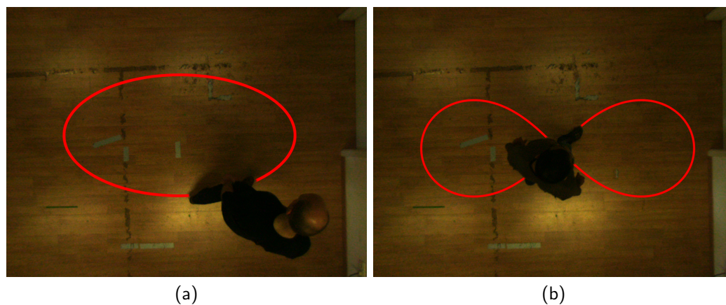
FIGURE 2.29: Schematic trajectories for the two sequences recorded for monocular pedestrian tracking evaluation, overlaid on camera images. The first trajectory (a) resembles an ellipse, while the second trajectory (b) resembles a Bernoulian lemniscate [169] ( i.e. eight-shape).
