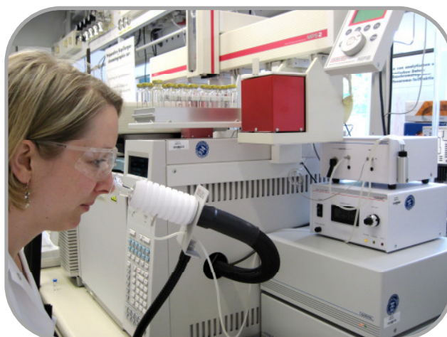
Figure 13: Gas chromatography-olfactometry (GC-O) with a sniffing port, where the eluted compounds can be directly smelled and evaluated by the assessor, in parallel with a flame ionization detector (FID).
