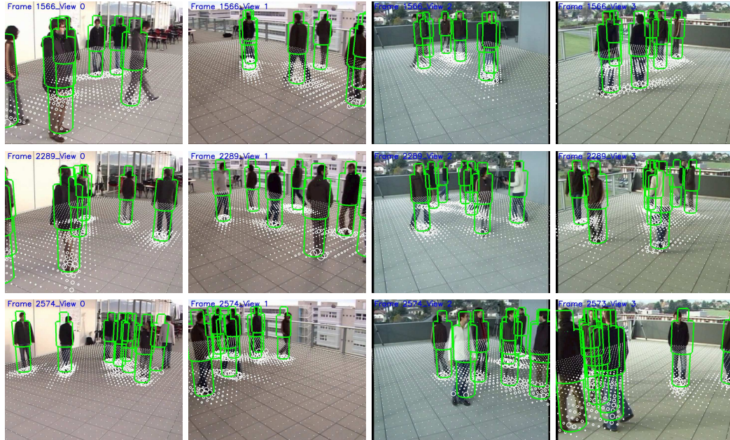
Figure 4.14: Detection results on the sequence of EPFL-Terrace. Every row shows a different frame, while every column displays different camera view. The likelihood grid maps of the finest level are superimposed onto the detection results, illustrating the likelihood for each detected person in corresponding frame.
