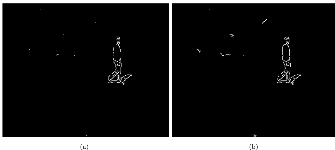
Figure 4.5: Illustration of the postprocessing result. (a) Edge map before postprocessing. (b) Edge map after postprocessing, the gaps are closed mostly within the unconnected edges.
