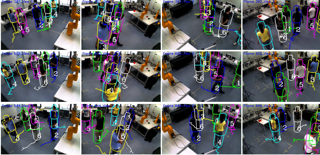
Figure 6.6: Tracking performance of our proposed approach on our own laboratory dataset with 6 targets involved, aiming to test the performance under crowded environment. Every row shows a different frame, while every column displays different camera view.
