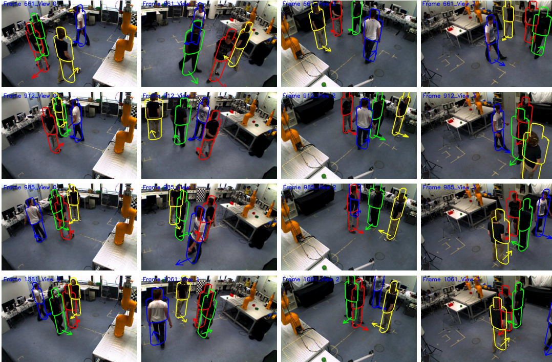
Figure 5.9: Human body orientation estimation results on the sequence of Laboratory 4 Targets, aim to evaluate the performance when target walking across others with very close proximity. Every row consists of views from four different camera views at the same time frame. The arrow indicates the orientation of the human body in 3D world space.
