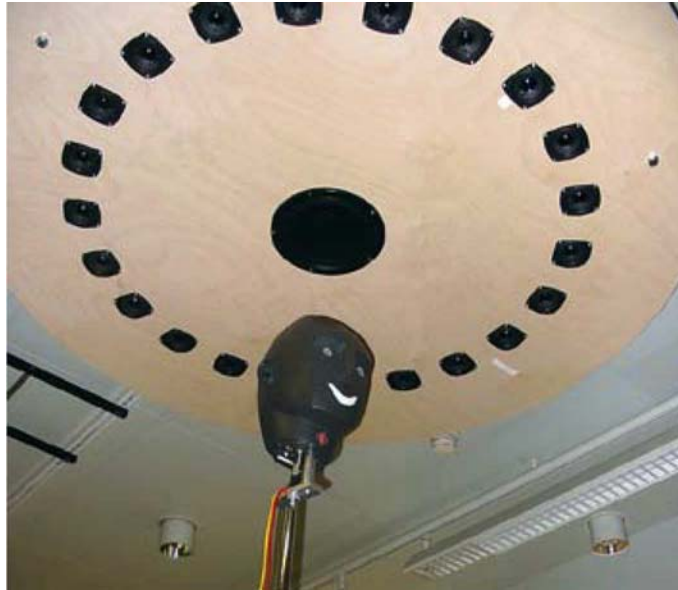
FIGURE 5. "Virtual headphone": Ring of 22 loudspeakers plus a woofer to project focused sources onto the ears using a kind of wave field synthesis (after Menzel et al. 2005).
