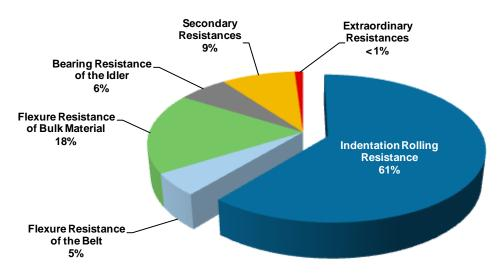
Fig. 5: Percental distribution of motion resistances of a long-distance horizontal belt conveyor [17]
