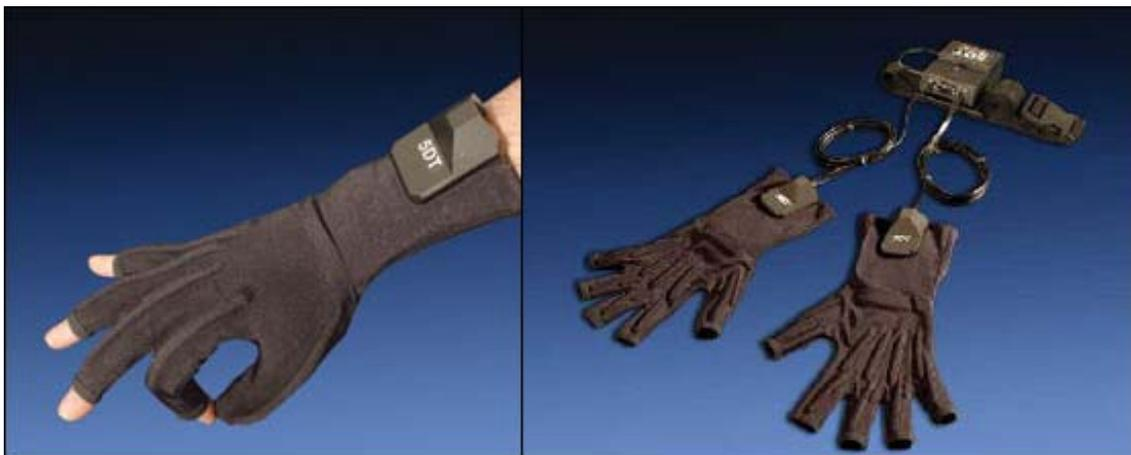
Abbildung 8-1: 5DT Data Glove / 5DT Ultra Wireless Kit [5dt-10]
