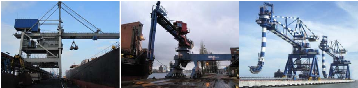
Fig. 6: Gantry Crane, Vertical Screw and Bucket Elevator for unloading coal from seagoing vessels.
