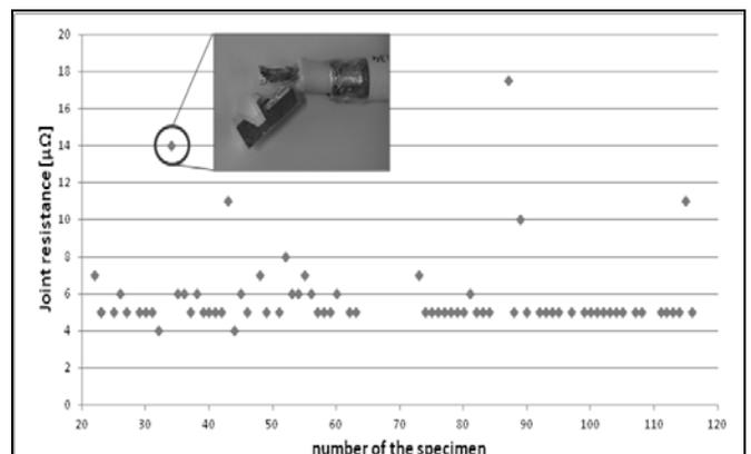
Figure 14: Electric qualification of ultrasonic welding
