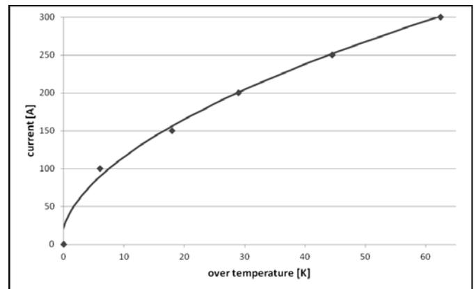
Figure 8: Ampacity of the LEIKO connector
