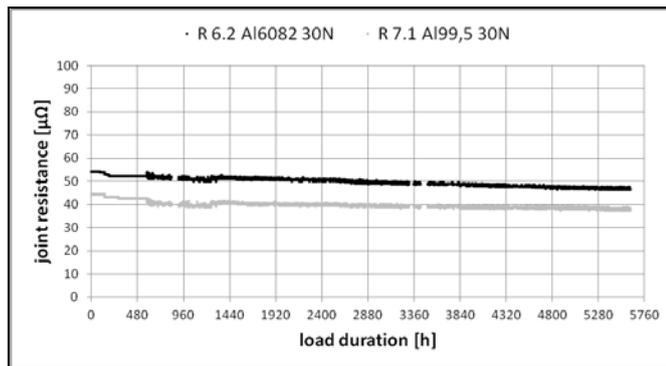
Figure 15: Joint resistance over time measured during long term thermal and electrical load
