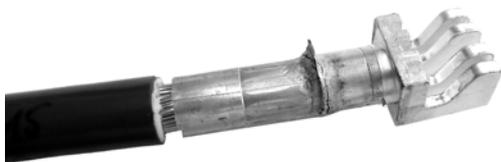
Figure 11: Resistance butt welded connector
