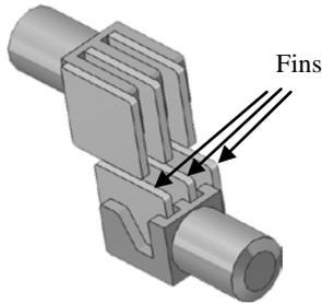
Figure 4: Protection against electrical shock hazard
