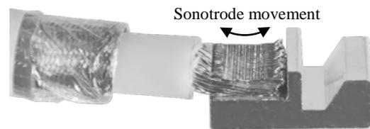
Figure 13: Ultrasonic welded connector
