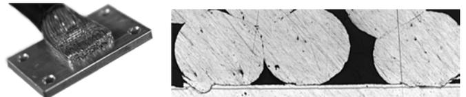
Figure 12: Ultrasonic welded cable
