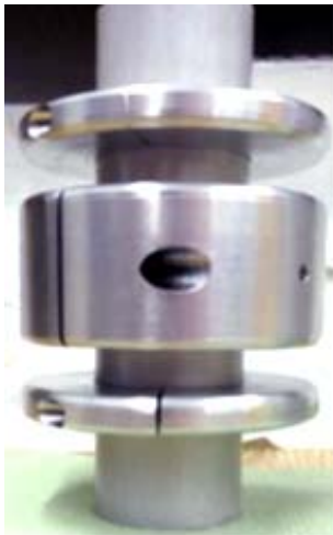
Figure 11 , left: Electrode configuration for the surface measurements. The cylinder surface (under the electrodes) is prepared with silver conductive painting in order to provide good electrical contact. Gap between the electrodes: 10 mm. Right: Currents measured on the surface of the cylindrical specimens at two different temperatures ( \vartheta = 60\text{ °C} and 100\text{ °C} ), recorded in a dry atmosphere temperature chamber. The blue triangle represents the measured current value of the bulk at \vartheta = 100\text{ °C} and E = 1\text{ kV/mm} .
