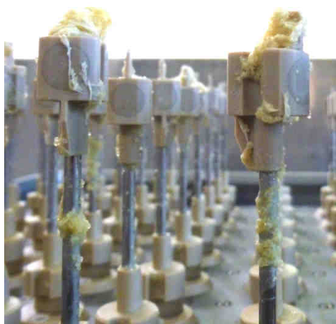
Figure 7.29 S-impellers after 5 h batch biotransformation using 64 \text{ g}_{\text{CDW}} \text{ L}^{-1} E. coli pET28NosT7FDH 3M , 400 mM (R)-carvone and 500 mM formate at a resin to substrate mass ratio of 4.
