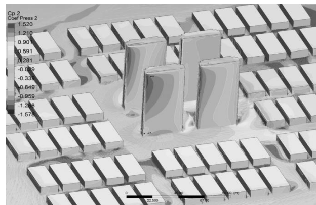
Figure 7: Concentration of higher C_p values zone close to the corner of the model building in southeast wind incidence
