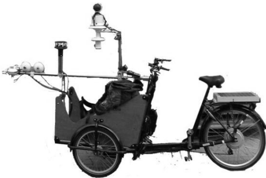
Figure 3: Cargo-bicycle equipped with micrometeorological measurement sensors
