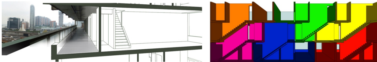
Figure 1: Robin Hood Gardens, one of some fifty housing schemes studied in London for the Masters programme in Sustainable Environmental Design. This iconic building designed by Alison and Peter Smithson in the late 1960s is now being demolished. Measurements and simulations performed for this scheme highlighted both the ingenuity of its complex interweaving of dwellings (coloured section, right) and the environmental weaknesses this built form and its "streets in the sky"(left) entailed [1].
