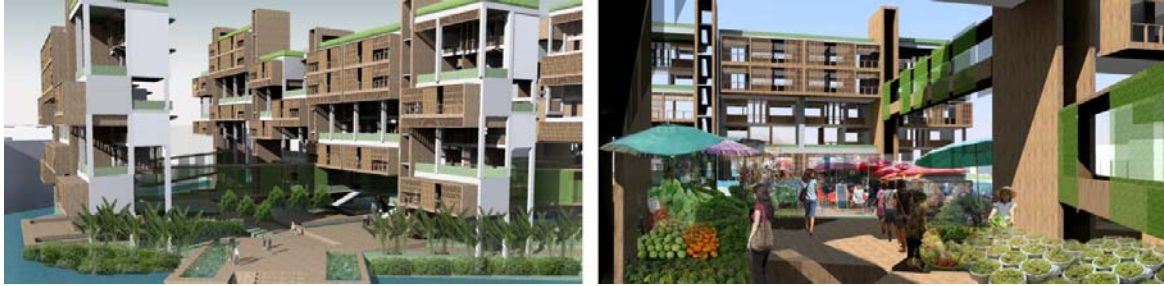
Figure 8 : This proposal for self-sufficient social housing eliminates the use of glass on its external elevations replacing them with a screen that is permeable to airflow and light while protecting from direct sun drawing inspiration from the life and built form of the Thai vernacular in Bangkok, Thailand, 13° 45 N 100° 29 E [10].
