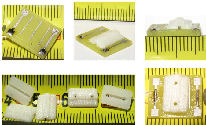
Fig. 5. Thermistors (diameter 0.36 mm) mounted on a board, canals to cover the thermistor and a thermistor covered with a plastic canal.
