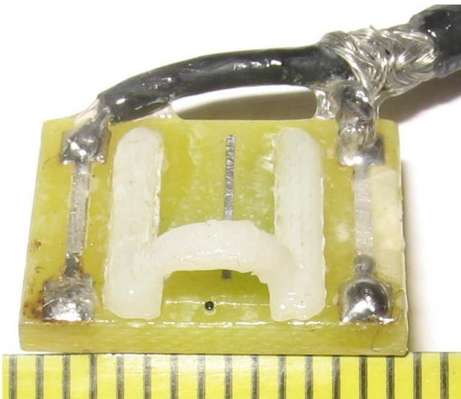
Fig. 4. The black thermistor (diameter 0.36 mm) sits under a protective bow. The yellow scale below indicates millimeters.
