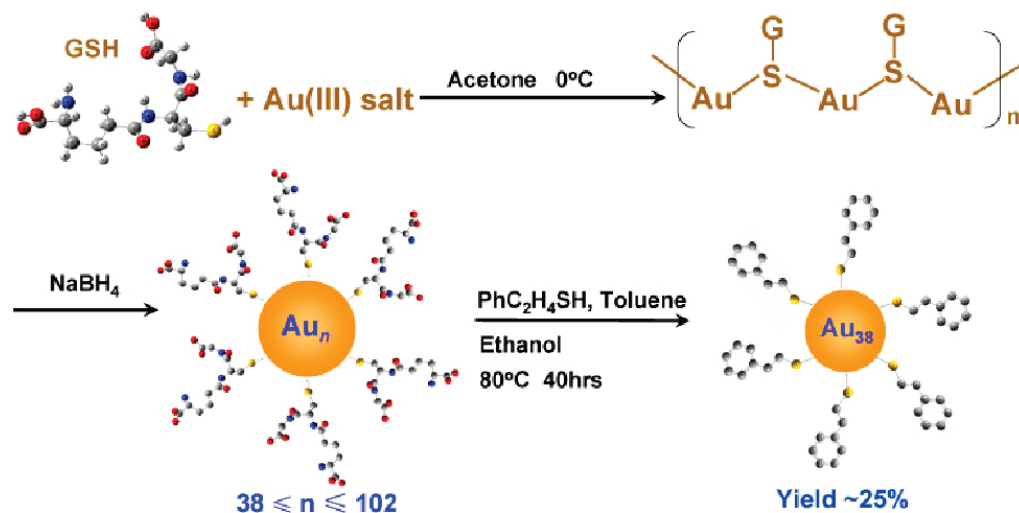
Scheme 9: A two-step procedure for synthesizing monodisperse \text{Au}_{38}(\text{SC}_2\text{H}_4\text{Ph})_{24} clusters in high yield. Reprinted with permission from ref. 96. Copyright (2009) The American Chemical Society.
