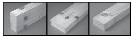
Figure 5. Presence of defects (knots) in a timber element.
