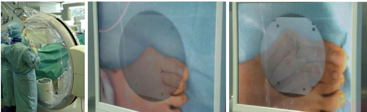
Figure 2.22: The images of the first surgery performed using the CamC system on July 02, 2009. The left image shows the CamC system setup in the OR. The last two images demonstrate that the primary surgeon uses the overlay image as a guidance to position the C-arm to acquire a desired X-ray image showing exactly the bone deformity of the toe.
