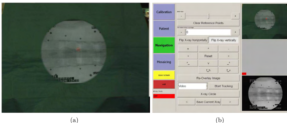
Figure 2.18: (a) The live video overlaid by the X-ray image shown on the LCD monitor; (b) The control interface of the CamC software shown on the touch screen .
