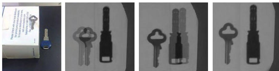
Figure 3.1: Illustration of the parallax effects in the panorama of stitching two X-ray images. From left to right, the first image shows the construction of two metal keys on two different parallel planes. The second image is the panorama generated using the transformation for the plane of the bigger key, and the third image shows the panorama generated using the transformation for the plane of the smaller key. The last image presents a parallax-free panorama generated by the X-ray source undergoing a relative pure rotation.
