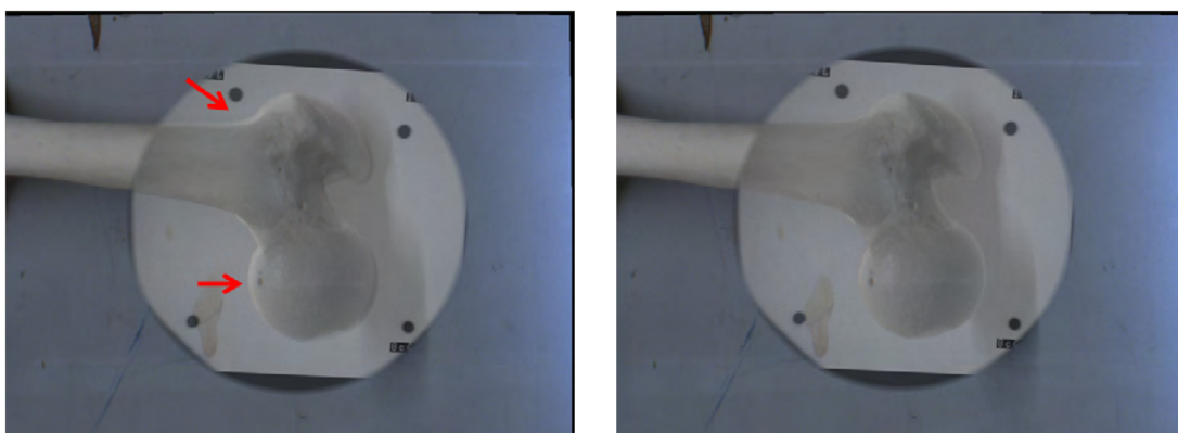
Figure 2.13: The left image shows the X-ray and video image overlay of the dry femur bone without applying the VDP method in the C-arm orientation of angular 60°. The right image shows the same bone with the VDP method used in the same C-arm orientation. The arrows indicate clear misalignments between X-ray and video images in the left image.
