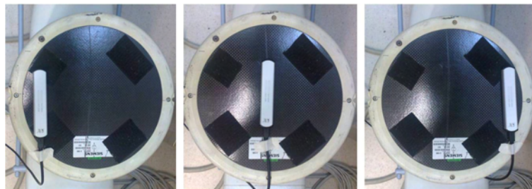
Figure 2.15: The positions of the Unfors Xi R/F Detector in our experiments. From the left to the right, they are position A, position B and position C.
