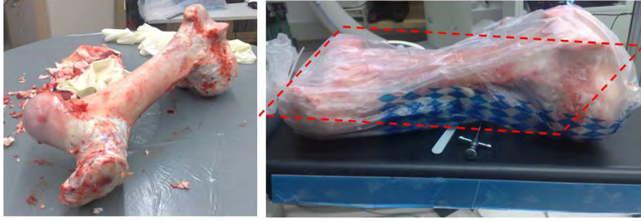
Figure 3.9: The left image shows a real cow’s femoral bone. The right image shows the setup for generating panoramic X-ray images of the real cow bone with two metal tools below.
