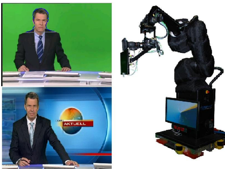
Figure 6.1: A virtual set for daily news broadcasting events. The upper and lower left pictures show the virtual studio. The right shows our robot camera system for broadcast automation. ( image courtesy: RTL Television Studio Köln, Germany, and Robotics Technology Leaders GmbH ).
