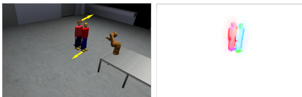
Figure 4.3: Optical flow processing results when the two targets are moving close to each other but in opposite directions
