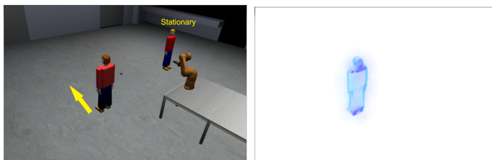
Figure 4.2: Optical flow processing results when one target is stationary and the other is moving
