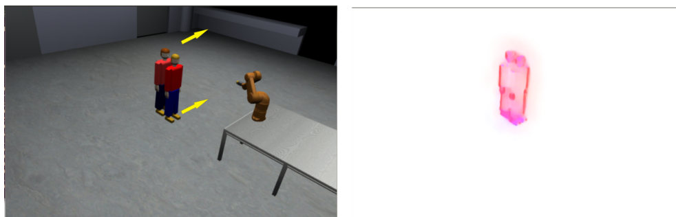
Figure 4.4: Optical flow processing results when the two targets are moving close to each other and in the same direction
