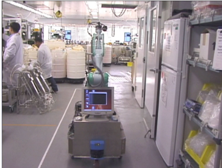
Figure 1.2: A mobile robot with an industrial arm in a bio-tech laboratory [1].
