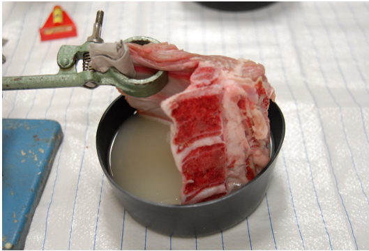
Figure 6.14: Embedding the lower part of specimen.
