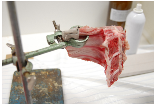
Figure 6.13: Fixation of specimen with the monopod.
