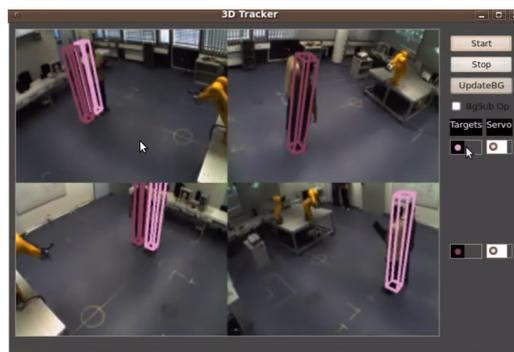
Figure 4.3: The figure illustrates how the system detects occlusion between targets.
