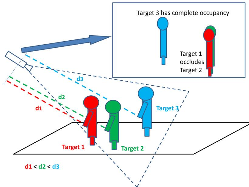
Figure 3.2: The figure illustrates the occlusion test system. The left part of the figure shows a scene in a camera view with 3 targets, where target 1 occludes target 2. The right part of the figure shows how the occlusion is detected by rendering the targets with respect to their distance from the camera. The target closest to the camera is rendered first.
