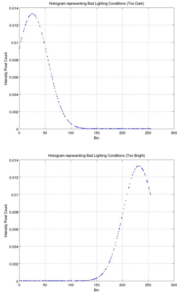
Figure 5.3: The figure illustrates bad lighting conditions by observing the histograms of the intensity channel.
