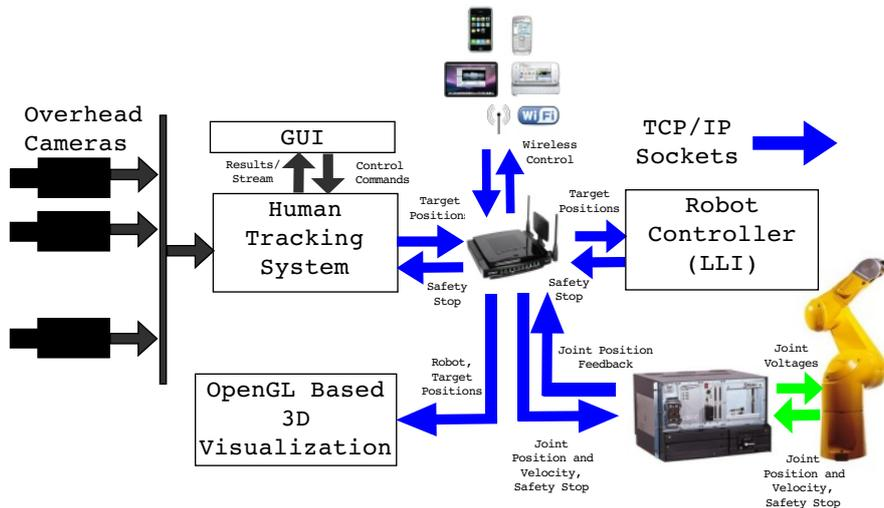
Figure 4.1: The figure provides the overview of the tracking system used in a real-world application for visual servoing of multiple targets in operational space using an industrial robot arm.
