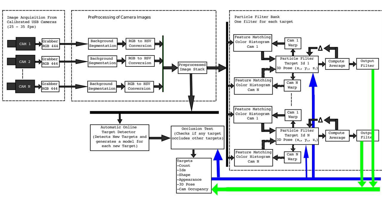
Figure 3.1: The figure illustrates the block diagram of the tracking system. It consists of the image acquisition module, target detection module, occlusion test module and the particle filter bank.
