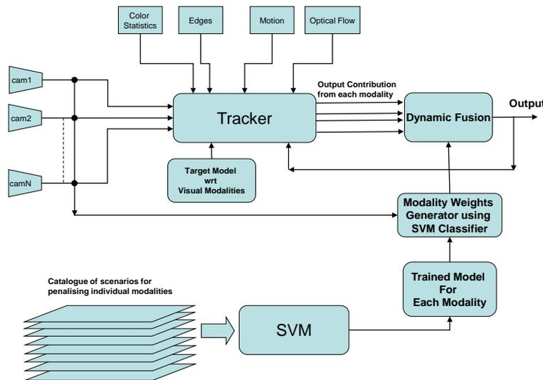
Figure 5.1: The figure illustrates the block diagram of the proposed intelligent multi-modal fusion module.
