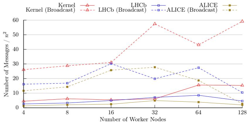
Figure 7.5: Number of messages divided by  $n^2$  with  $n$  worker nodes. Our customized message dissemination requires several factors less network packets than a naive broadcast.
