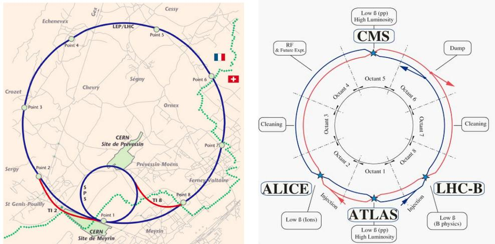
Figure 2.1: Left hand side: the perimeter of the Large Hadron Collider (LHC) and the transfer lines to the *SPS* pre-accelerator embedded in a map of the area (source: L. Guiraud, CERN public picture collection). Right hand side: a schematic image of the LHC as presented by Evans and Bryant [EB08].
