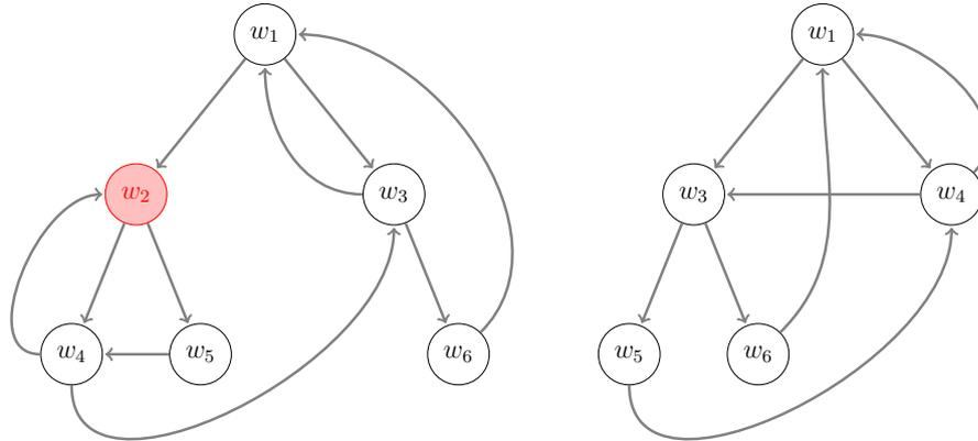
Figure 6.9: *Left hand side:* A 6 node LDI graph with fan-out 2. If worker node  $w_2$  fails in the middle of state dissemination, worker nodes  $w_4$  and  $w_5$  become unreachable from worker nodes  $w_1, w_3$ , and  $w_6$ . *Right hand side:* As soon as worker node  $w_2$  is detected as dead, the worker nodes re-organize the dissemination graph to an LDI graph with 5 nodes.
