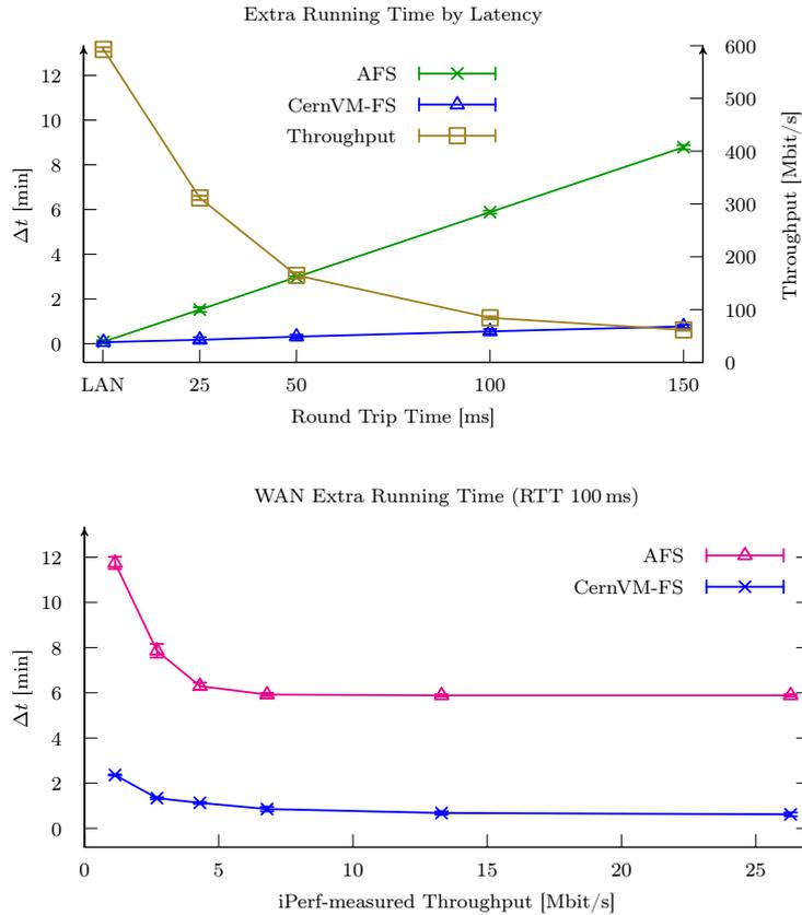
Figure 7.8: Time penalty as a function of latency and bandwidth comparing AFS and CernVM-FS to local storage for running the ROOT benchmark *stressHepix*. With standard window sizes of 16 KiB the TCP throughput is directly affected by latency. A round trip time of 100 ms corresponds to observed parameters between a worker node running on Amazon EC2 (U.S. East Coast) accessing services located at CERN.
