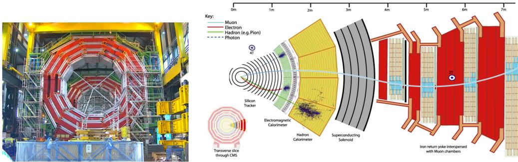
Figure 2.2: Left hand side: The profile of the CMS detector before final assembly (own photography). Right hand side: a schematic profile of the CMS detector (source: CMS public web site).
