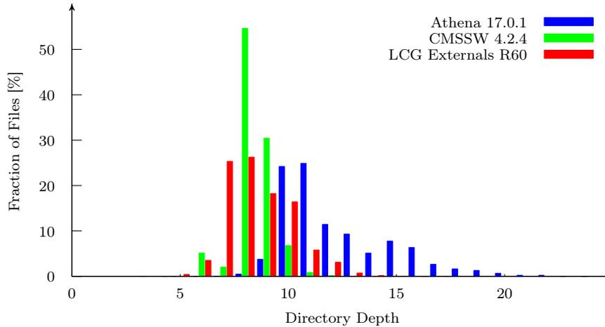
Figure 4.5: Fraction of files on located at a certain directory level. Counting starts with the highest directory under the responsibility of the collaboration, i. e. there are no artificial leading levels such as `/usr/local`.
