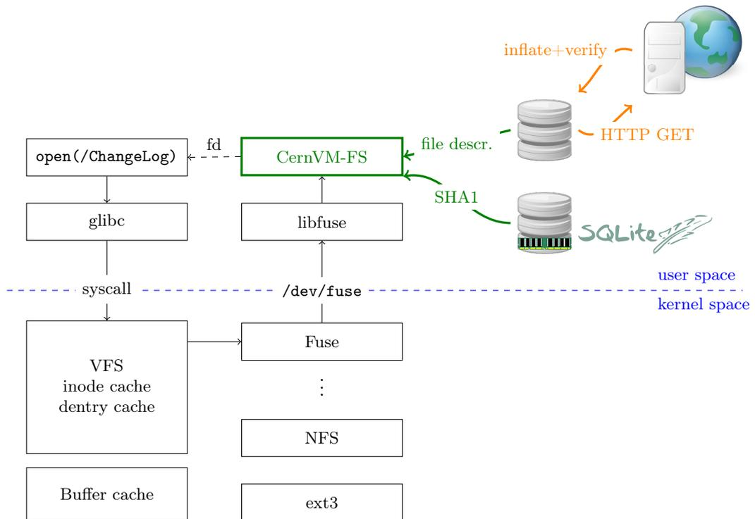
Figure 7.1: Process of opening a file. CernVM-FS resolves the name by means of an SQLite catalog, which is prepended by a memory cache. Downloaded files are verified against the cryptographic hash of the corresponding entry in the file catalog. The `read()` and the `stat()` system calls can be entirely served from the in-kernel file system buffers.
