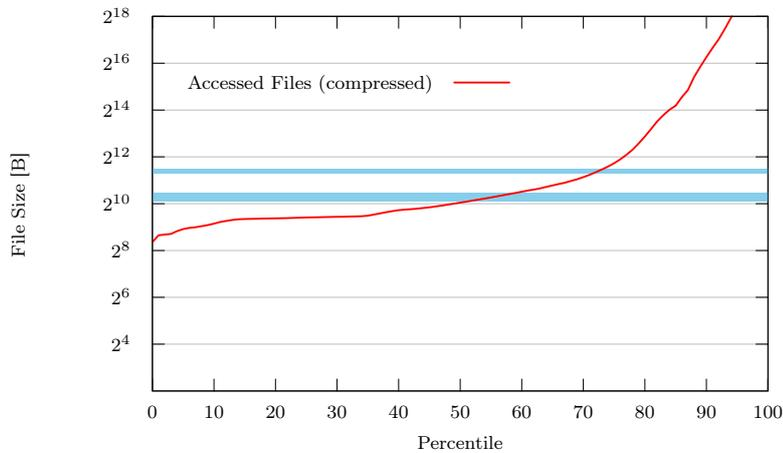
Figure 7.2: Cumulative size distribution of requested files. Files are DEFLATE compressed. The sample consists of operation traces over 1 month comprising 14 million requests. The blue bars show the range from 1092 B to 1422 B and from 2514 B to 2844 B, respectively. The height of the bars correspond to the observed average HTTP header size of 330 B.
