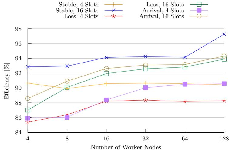
Figure 6.8: Efficiency in case of large and sudden changes in the number of available worker nodes. The configurations refer to the total number of worker nodes during a simulation run, i. e. before the loss of nodes and after the arrival of nodes.
