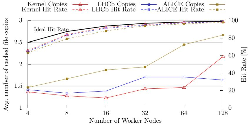
Figure 7.4: Redundancy factors of the distributed memory cache. The redundancy factor specifies how many times a file is requested from a Stratum 1 server. The redundancy factor in conjunction with the number of worker nodes specifies the cache hit rate. For  $n$  worker nodes the ideal cache hit rate is  $(n - 1)/n$ .
