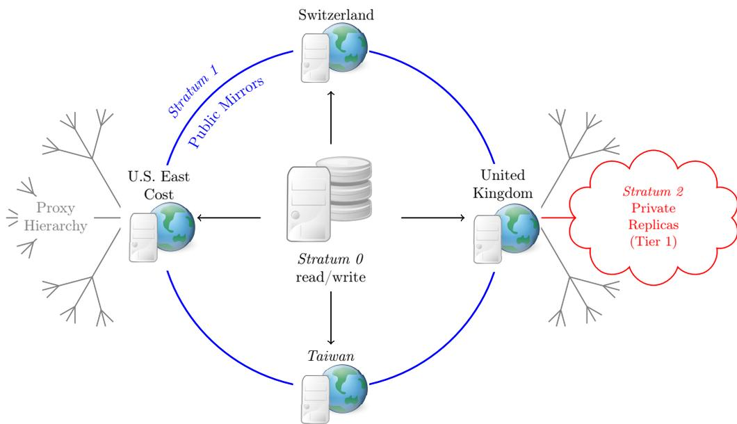
Figure 7.3: HTTP content delivery network: Replica servers are arranged in rings (Stratum 0 – Stratum 2). One protected r/w instance feeds several reliable, public, and globally distributed mirror servers. A distributed hierarchy of web caches fetches content from the closest public mirror server. The public mirror server can in turn be a master for private mirror servers, which might be demanded by large computing centers.
