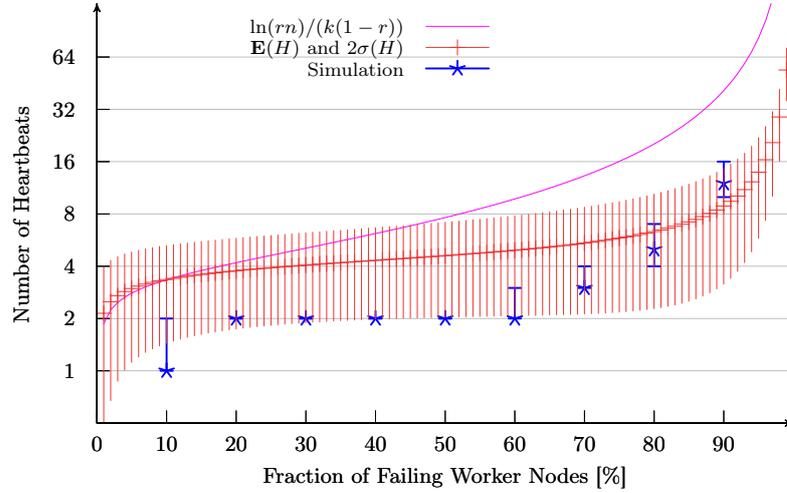
Figure 6.10: Dead worker node detection performance in number of heartbeats required to detect all failed worker nodes for 4096 nodes. For each failure rate, the failing worker nodes are chosen at random. Each simulation step is repeated  $10^4$  times.
