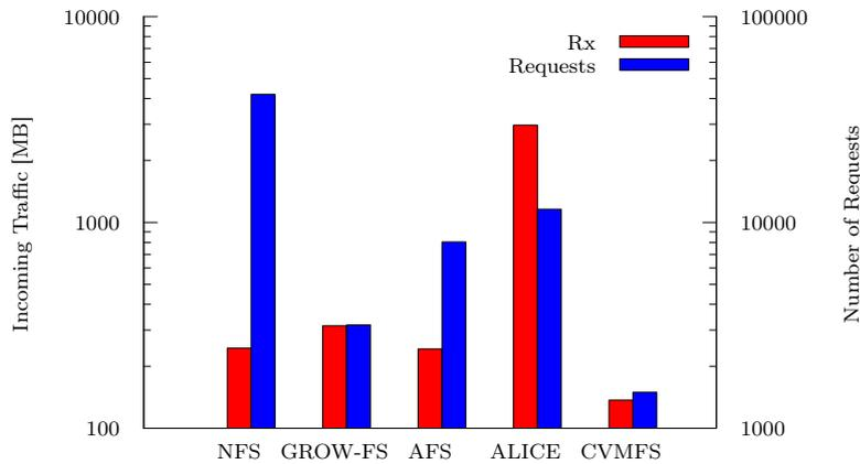
Figure 7.7: Incoming traffic and number of requests for running the ATLAS event viewer. NFS and AFS benefit from accessing only blocks of files. CernVM-FS benefits from compression and HTTP keep-alive connections. ALICE installation framework requests are usually distributed among the site’s worker nodes.
