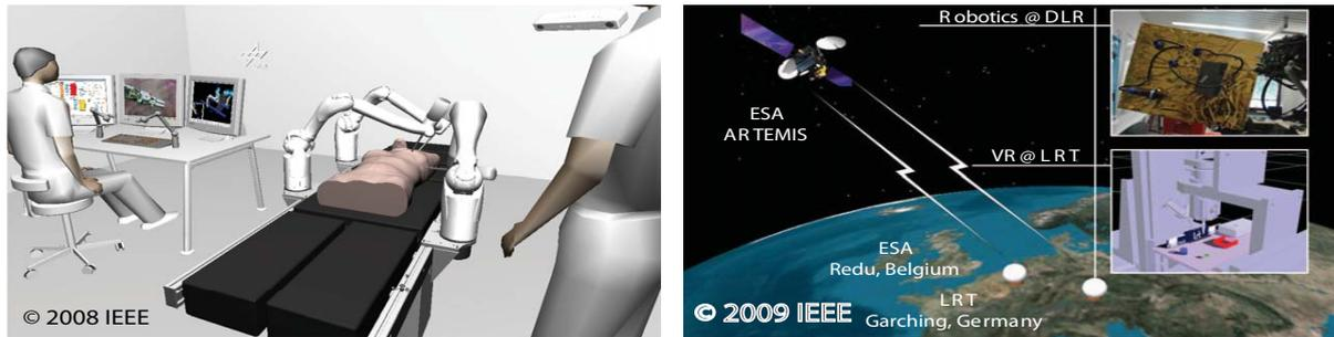
(a) DLR's telesurgery system. Image courtesy of [54]. (b) TUM's and DLR's joint on-orbit-servicing experiment. Image courtesy of [156].
