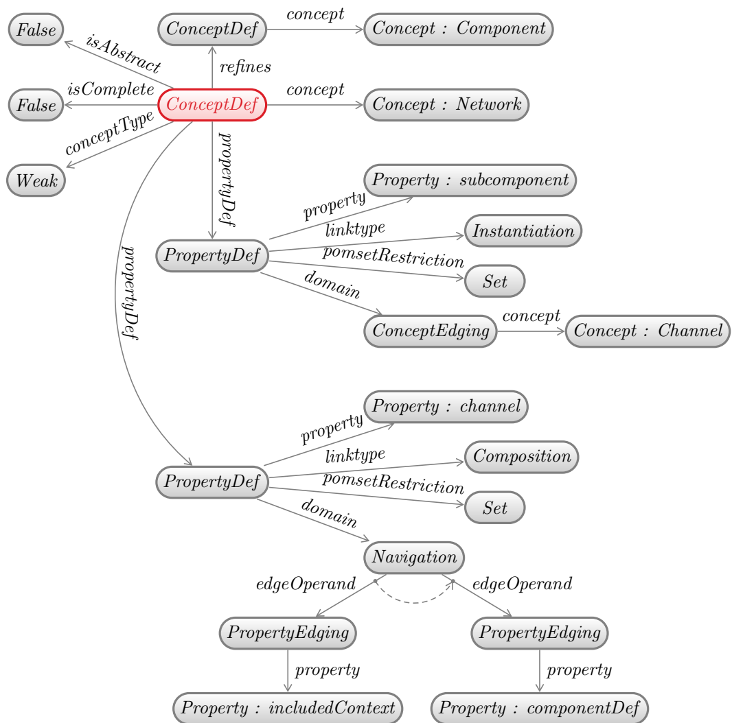
Figure 7.15.: Example: specification of the concept Network in the form of an abstract word
