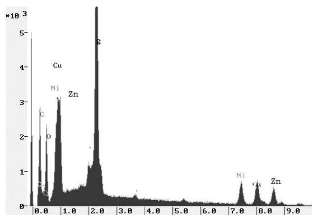
**Fig. 2-12.** EDS spectrum of the precipitate of R2 experiment
