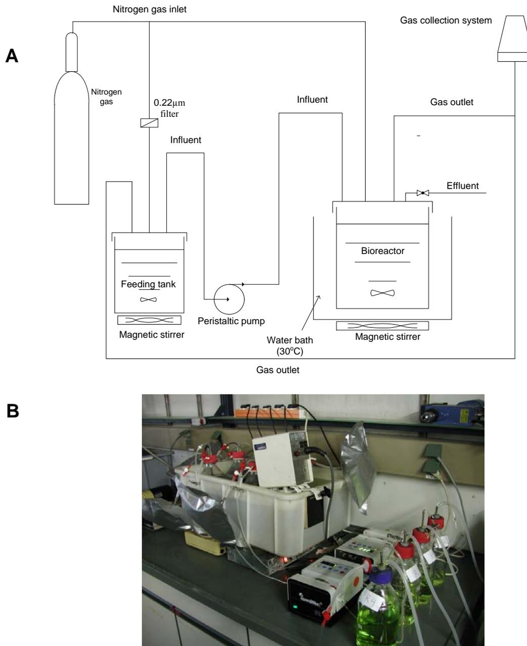
**Fig. 2-2.** Semi-continuous stirred tank reactor (A) configuration, (B) photograph
