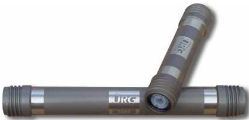
Figure 3-5. Three channels annular denuders used in this study.
