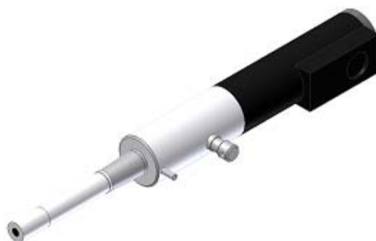
Figure 3.1-1: Drawing of a rotating disk electrode including shaft and electrical motor.
