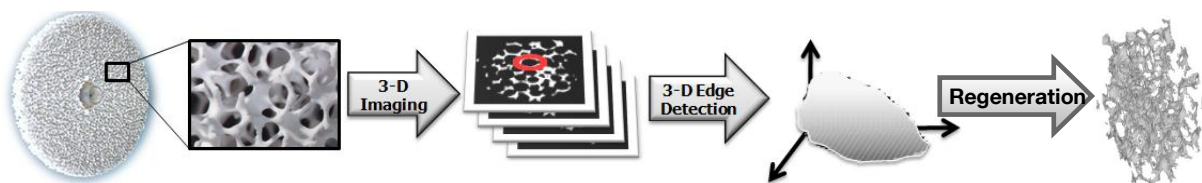
Figure 2.21: From the Micro-CT images 430 hundred 2-d binary edge images are assembled forming a 3-D binary file of the scaffolds.
