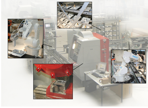
Figure 5. The hardware setup for experimentation, showing storage, transport, robot and machining components.
