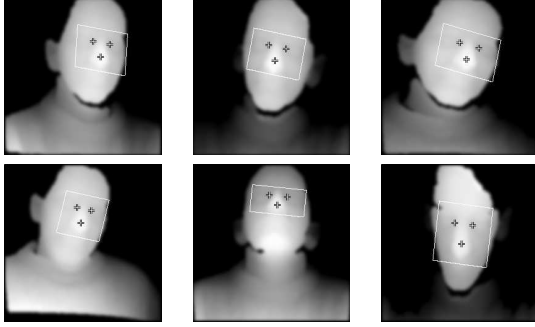
Fig. 5. Result of the feature detection, crosses denote eye corners and nose tip, the region of the best hypothesis found by the PCA-based classifier is boxed, from upper left to lower right: neutral , smile , laugh , random , look up , look down .
