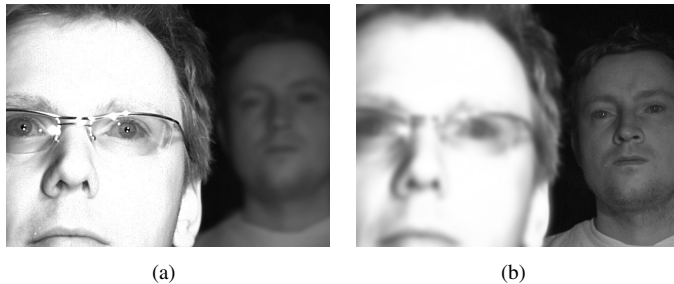
Fig. 6. Example for multiuser gaze tracking. For this images, we used a 16 mm optic with integrated liquid lens. One user was positioned at a distance of approx. 0.7 m and the second user at a distance of approx. 1.7 m. (a) shows the camera image focusing the front face, while (b) shows the camera image focusing the farther face.
