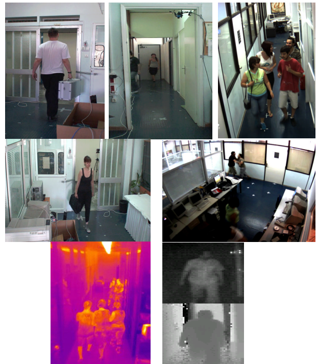
Fig. 1. Captured images of different narrow aisles, one entrance area with a larger door and one open area. Sensors used include video (top 5 images), thermal infrared (lower left) and a PMD device (lower right).
