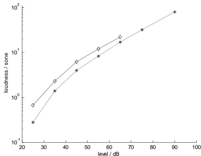
**Figure 1:** Loudness of pink noise as a function of its overall level. Rhombs connected by dashed lines represent loudness data given in ANSI S3.4-2007; stars connected by dotted lines indicate loudness data calculated according to DIN 45631 (1991).
