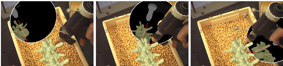
Figure 5.3: Mirror is rotated around the operation site to check the position of the drill canal. Box was filled with peas to simulate the restricted view on the operation site.
