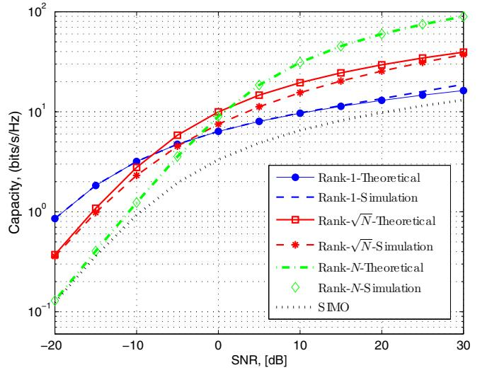
Fig. 4. Analytical and simulated capacity of three different LoS MIMO configurations against the SNR ( $N = 9$ ).
