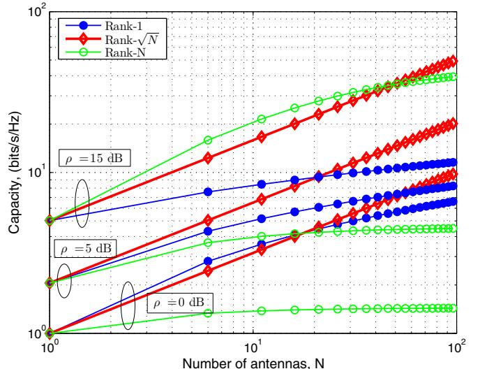
Fig. 3. Ergodic capacity for different MIMO configurations against the number of antennas  $N$  ( $\gamma = 1$ ).
