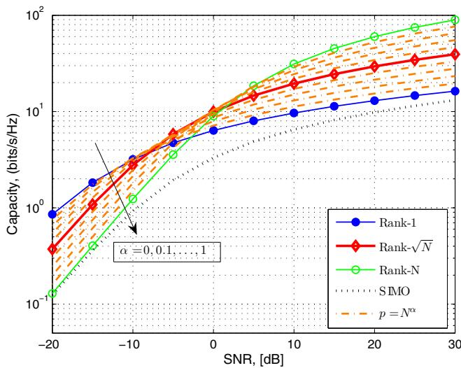
Fig. 2. Ergodic capacity for different MIMO configurations against the SNR ( $N = 9$ ,  $\gamma = 2$ ).
