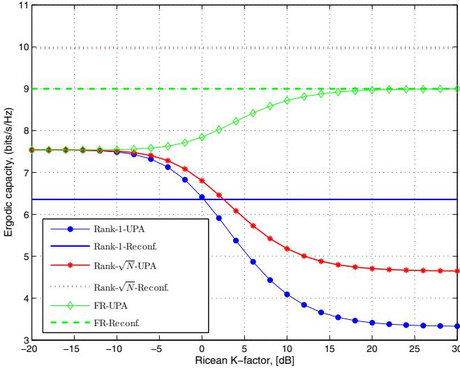
Fig. 5. Ergodic capacity of three different LoS MIMO configurations against the Ricean  $K$ -factor ( $N = 9$  and  $\rho = 0$  dB).
