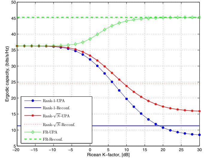
Fig. 6. Ergodic capacity of three different LoS MIMO configurations against the Ricean  $K$ -factor ( $N = 9$  and  $\rho = 15$  dB).
