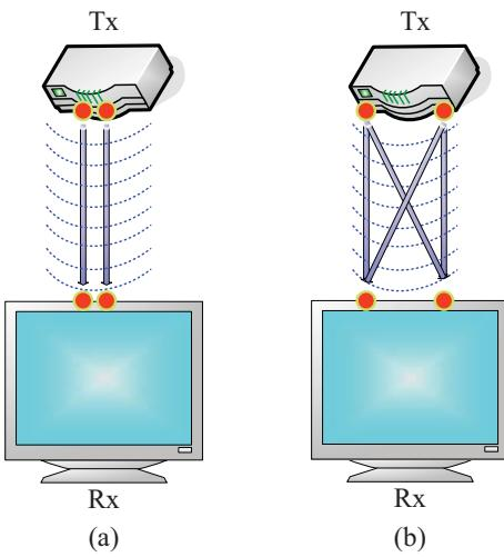
Fig. 1. Schematic illustration of (a) conventional and (b) optimized MIMO systems in LoS. The former configuration offers minimum multiplexing gains due to the high correlation between the LoS responses whereas the latter delivers orthogonal LoS subchannels.
